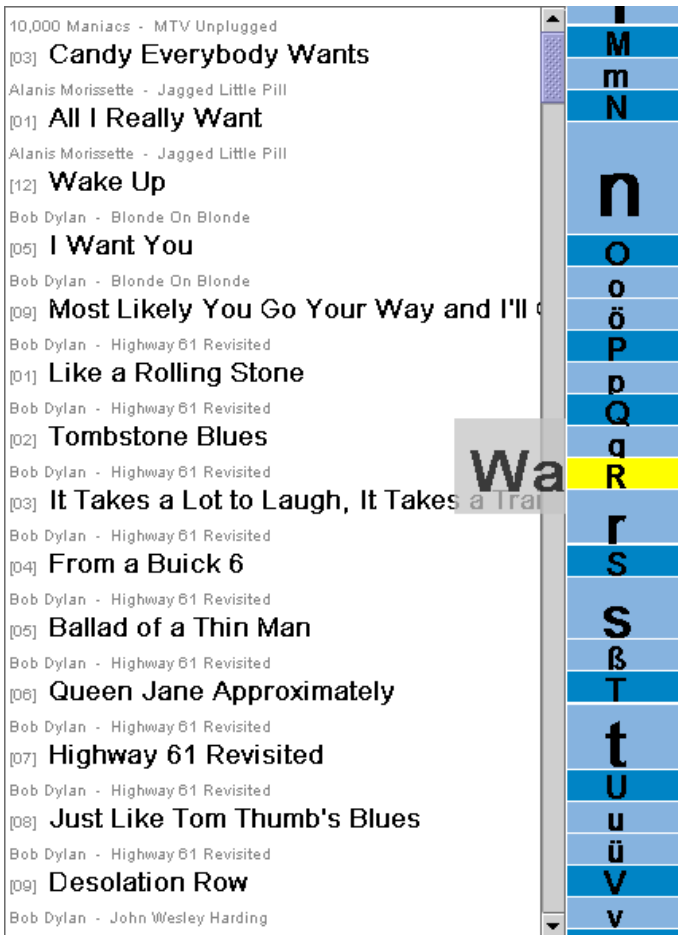
Figure: EnChoi is following the one-handed interaction paradigm, as operations are designed to allow a touchscreen text input with the bare thumb of the same hand that holds the device. Users can slide a letter ribbon up and down, whereby language statistics control for the size of the individual letter fields. By sliding to the left, the letter is entered (or removed again by sliding to the right). The screenshot shows a text search for 'Watchtower' in a music player application, two letters have already been entered. The database is incrementally searched and the list being updated accordingly.
