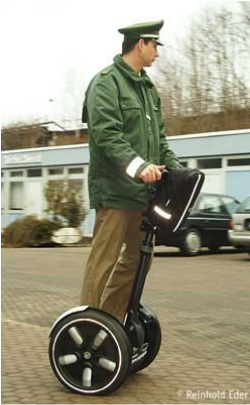
Figure: The Segway PT is an electric energy powered vehicle that is operated by slanting towards the intended direction. leaning forward results in an acceleration, leaning backward decelerates/halts. Leaning to the left results in a left turn etc.
